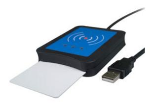
The Elatec TWN4 contact and contactless reader is a flexible and intelligent desktop USB device that is capable of reading and writing a wide range of contactless and RFID cards and tags, operating at both 125KHz and 13.56MHz, as well as any ISO 7816 contact smartcard via the built in card slot.
